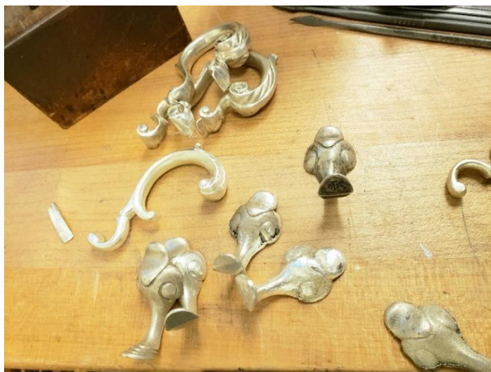
George's castings in various stages of completion. These will be used for cup handles and footings.
