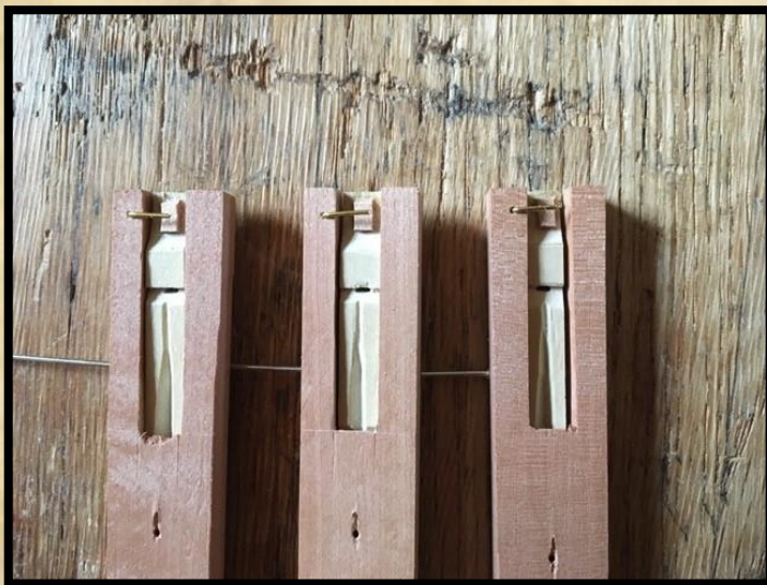
Staples for Jack Mechanism installed by Ed
