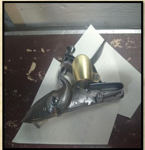
Polished Short Land Pattern Lock.jpg -- "A Short Land Pattern Service Musket lock recently serviced and polished to bring it back into good working order."
