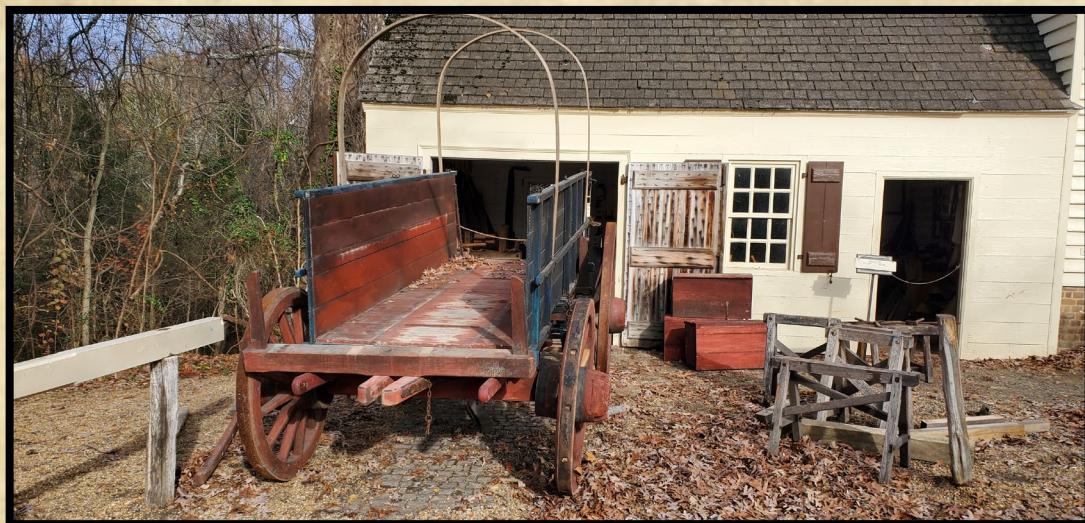
Fore under-carriage installed on Wagon.
