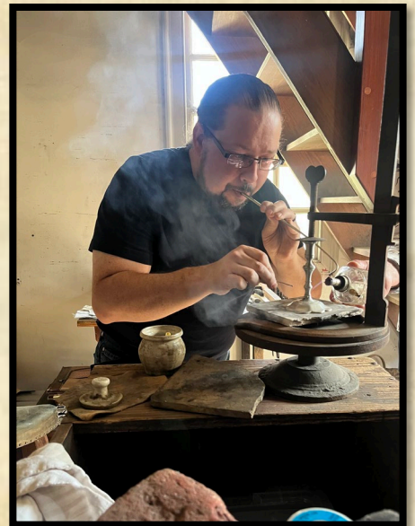
Drew blowpipe soldering his taper stick.
