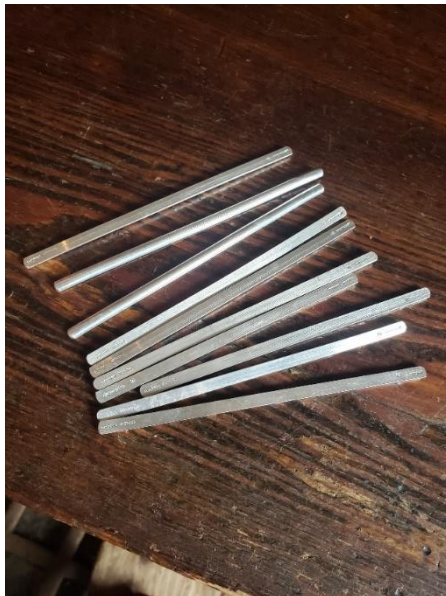
George's bracelet blanks made from hand cast and drawn ingots
