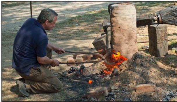
Colonial Williamsburg journeyman blacksmith Steve Mankowski pulls a "bloom" out of a small furnace used for smelting iron called a bloomery.
