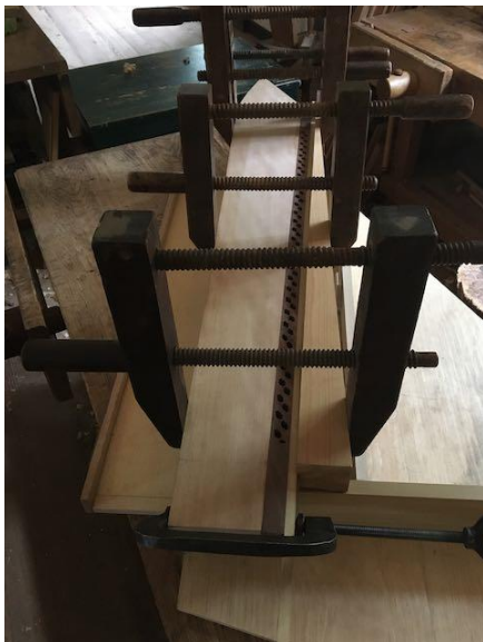
Gluing soundboard support liner to jack guide
