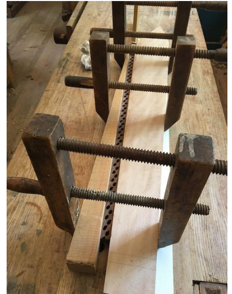
First veneered piece installed and finished (left). Full front mechanical assembly complete (center). Gluing jack guide to tuning wrist plank (right).
