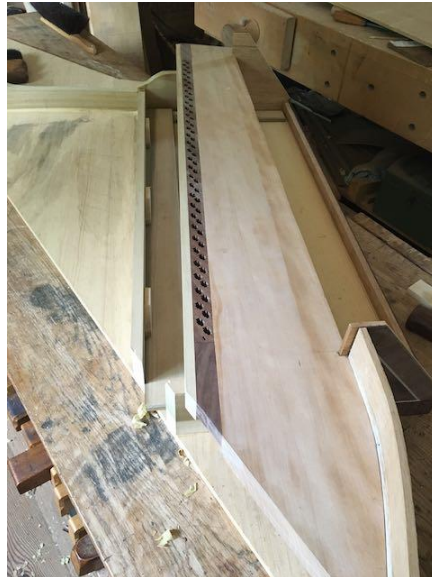
First veneered piece installed and finished (left). Full front mechanical assembly complete (center). Gluing jack guide to tuning wrist plank (right).
