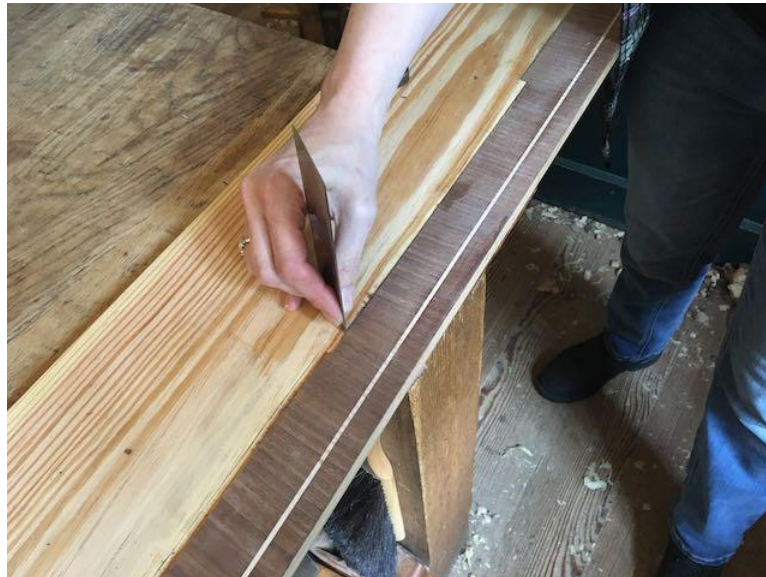
Trimming veneer back for later fittings
