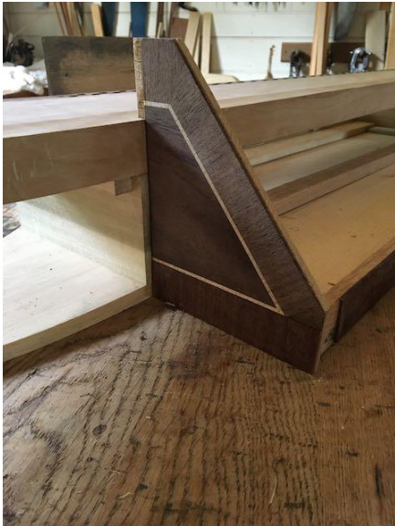
First veneered piece installed and finished (left). Full front mechanical assembly complete (center). Gluing jack guide to tuning wrist plank (right).
