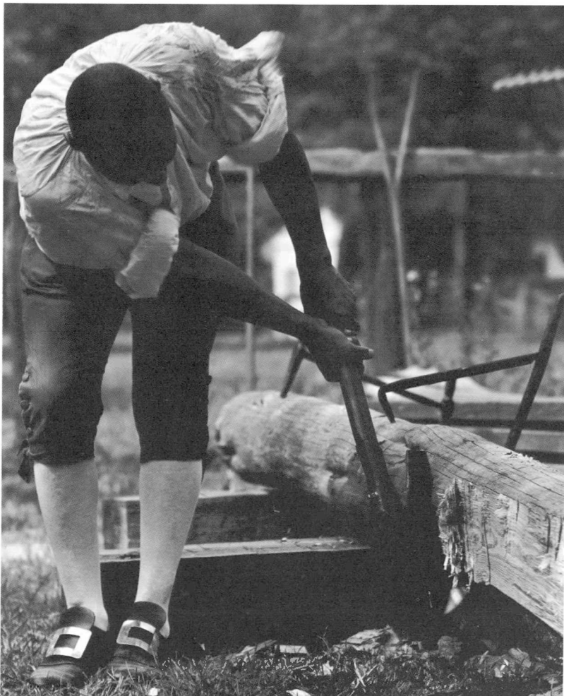
◀ Rough carpentry; hewing a log with a broad axe.
