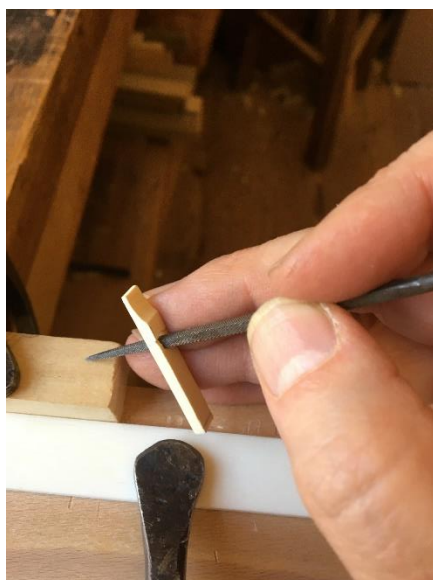
Smoothing the Mortise with Square Needle File
