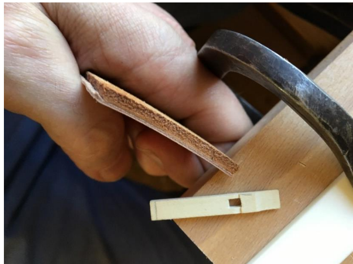
Leather laminate and jack tongue with sleeve hole
