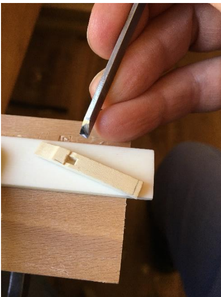
Chiseling mortise for leather plectra
