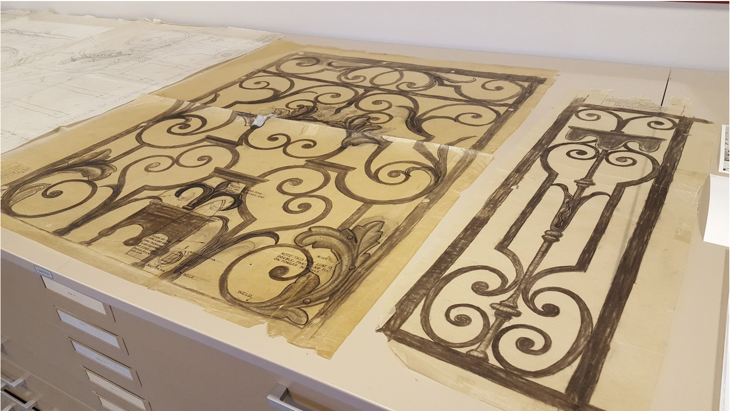
Full-scale drawings of ironwork details for a balcony on the Governor's Palace by Perry, Shaw & Hepburn, 1932.
