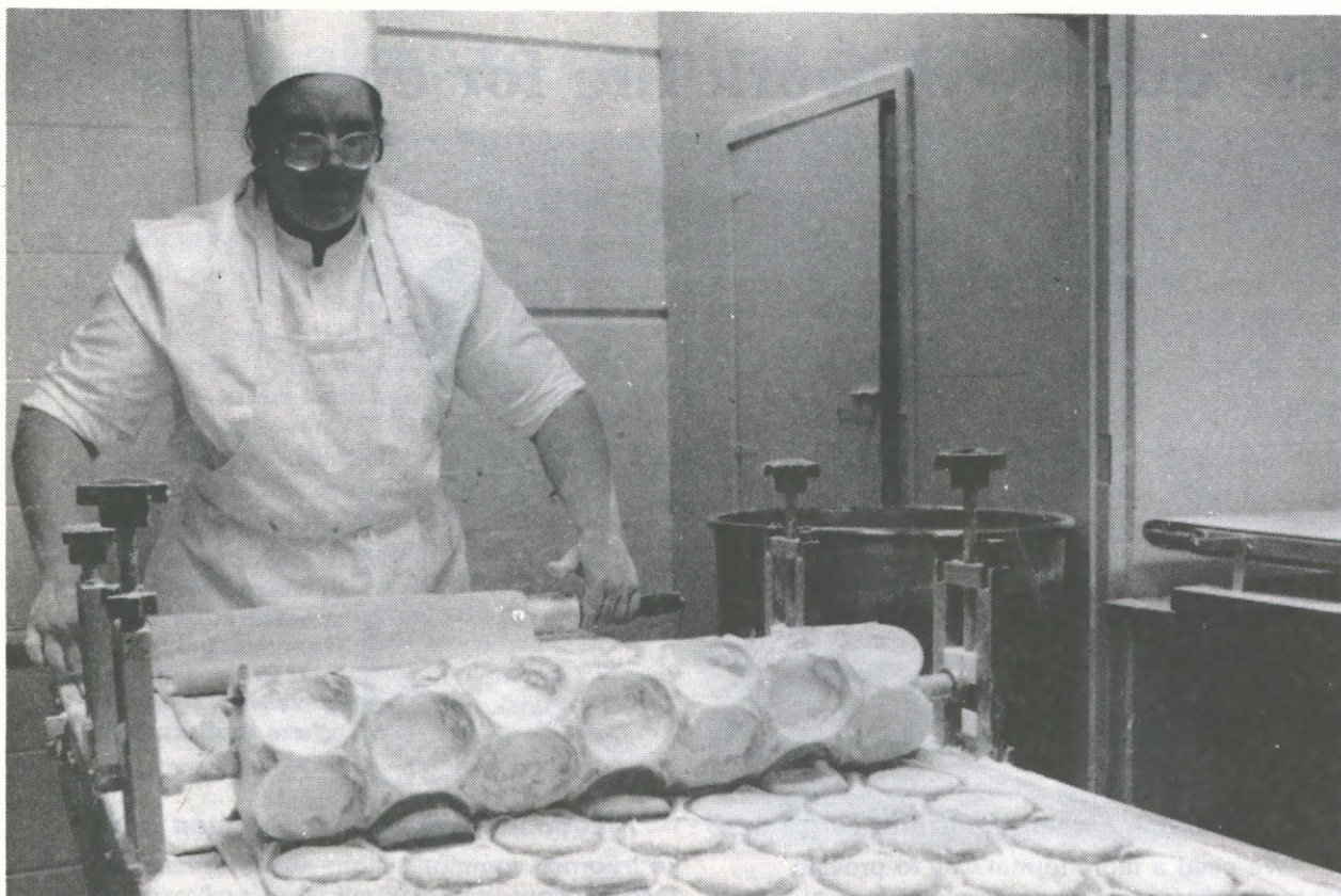
THE 'COOKIE CUTTER MACHINE', operated by Vicki Broshear, allows the Commissary to make up to 4,000 cookies per hour. Heidi Moore
