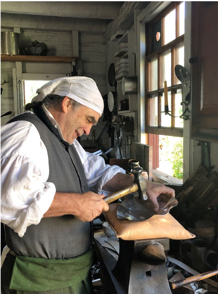
Steve starting to raise the shape of the lid in the morning.
