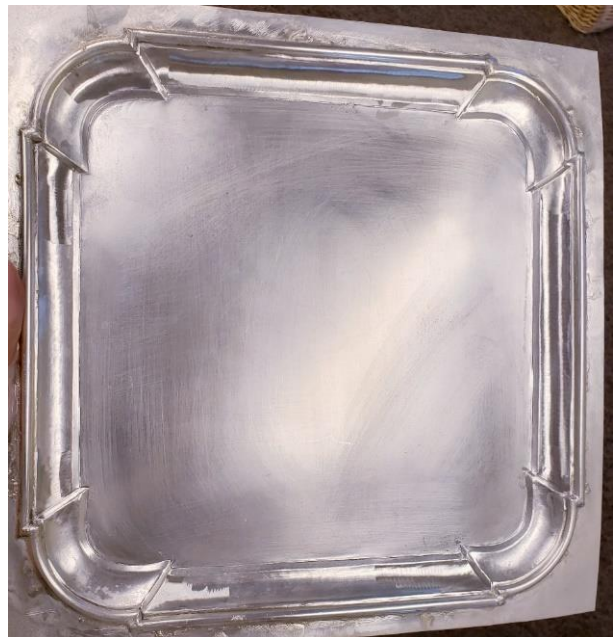
Bobbie's tray, soldered and ready for filing and stoning
