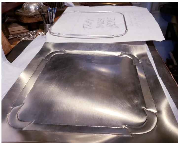
Chris' tray, the rim is soldered together, and the body of the tray is being chased in.
