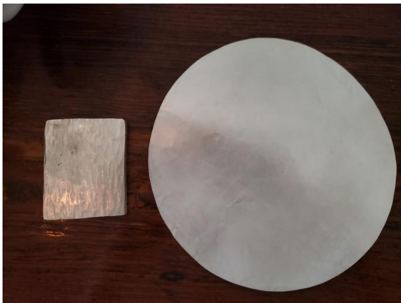
Left: One half of the ingot Megan cast. Right: The other half hammered into sheet, cut into shape, and currently being planished.
