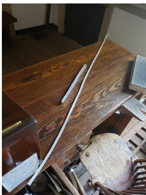
One of George's in-progress ingots on the left, the finished one on the right is ready to be cut into spoon blanks.
