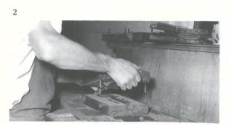
Above, Dan removes the top half of the flask which contains the desired mold. The master is shown at the bottom. Half of the mold is now complete. In this case Dan is preparing to cast a small taper stick, identical to one in CW's Department of Collections.
