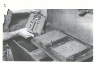
In the above picture one may compare the two molds Dan has made from the master which he is holding. The master may now be set aside for use again and again. Take note of the vertical cylindrical object which is located between the two halves of the taper stick. This object is referred to as a gate or sprue.
