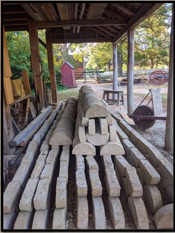
Sundried coping bricks taking shelter in the saw house.
