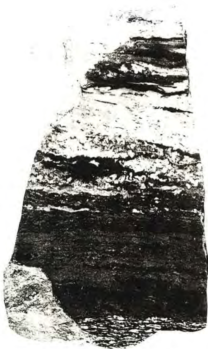
Polished surface of portion of vein-filling, Cranberry mine, Cranberry, N. C., showing association of ore with hornblende. The light bands are epidotized pegmatites, the black mineral is hornblende, and the gray one, in the lower part of the figure, is magnetite. The mixture of magnetite and hornblende is the ore. At the bottom of the figure is a small bit of epidote-hornblende gneiss. (Natural size.)
