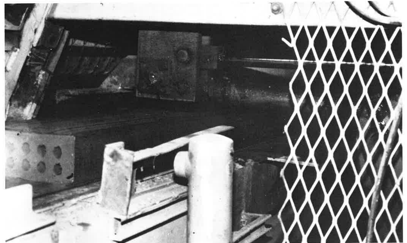
Manufacturing innovations are shared with the industry. Here a clay column moves toward the wire cutter.
