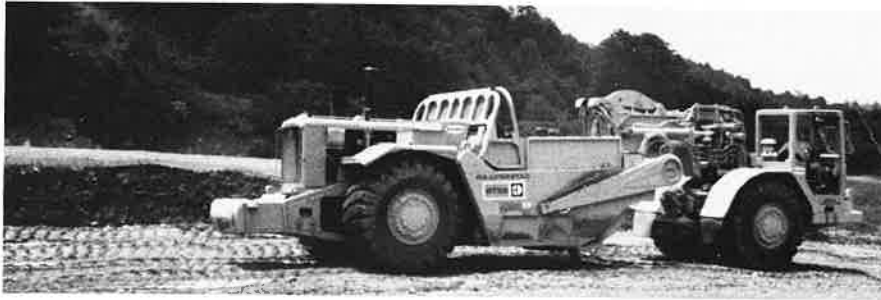
General Shale mines and stockpiles its own raw materials; here, a scraper works its way through a cut in one of the firm's pits.
