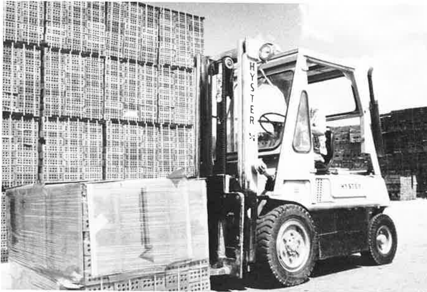
Forklifts remain a staple of any brick operation. Here one of General Shale's dozens of forklifts moves a pallet of brick into storage before being loaded on a truck for transit to a dealer.
