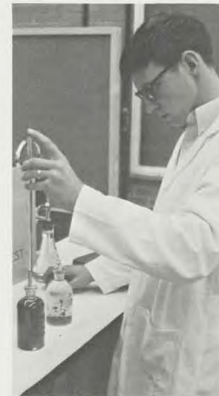
Student Wayne Hyatt runs a dissolved oxygen test on a stream sample.
