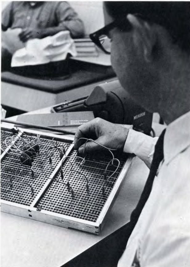
Mr. Cameron shows how to program a punch board for a business machine.
