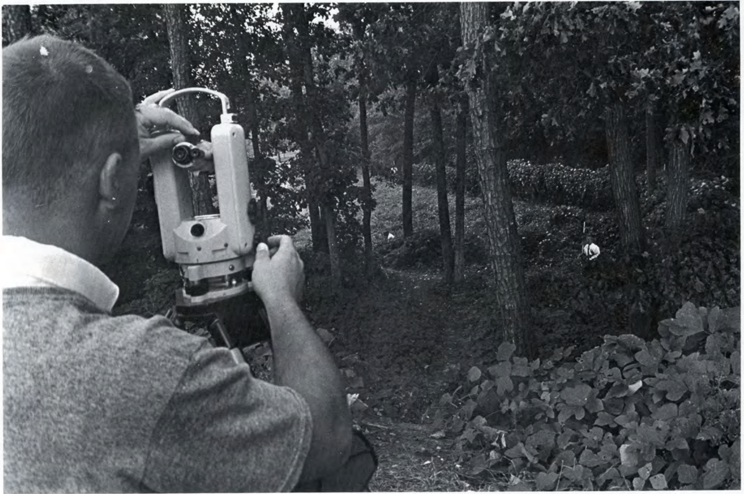
Civil Tech students gain practical experience in using a transit theodolite.
