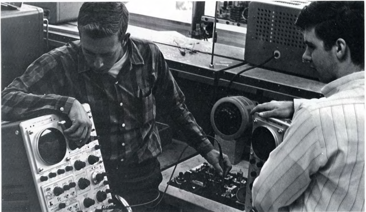
Larry Collier and Wayne Wiggins, Electronics II, use a Tektronix Type 545B Dual Beam Oscilloscope and Tektronix 575 Curve Tracer to examine transistor characteristics and determine their dynamic parameters in an operational transistorized superheterodyne AM Radio they have assembled.
