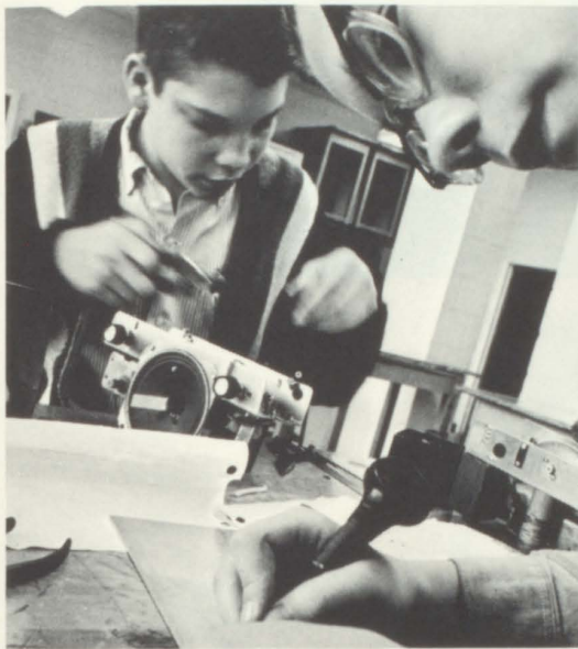
Electronic students construct a stereo amplifier as a quarter project.
