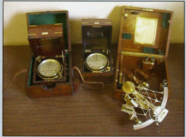
The marine chronometers on the left are precise timekeeping devices used in determining longitude by incorporating celestial navigation. The sextant on the right is used to measure, among other things, latitude, by determining the altitude of the sun or other celestial objects.
