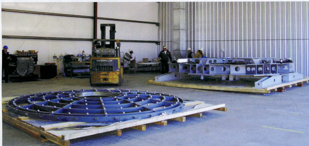
The mirror simulator (foreground) and cell (background) in the hangar at the Flagstaff airport before being turned over.
