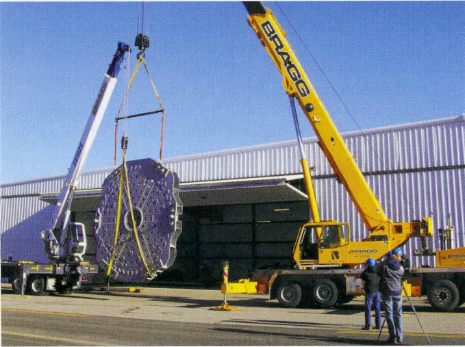
Precision Heavy Hauling turns over the DCT primary mirror cell at Flagstaff's Pulliam Airport in January.
