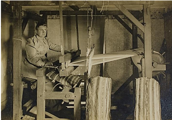
51. Granville, four post barn loom of mortise and tenon construction. Photograph, c. 1910, "Nelsie Harger Sheets at her loom in Aunt Eliza's attic over the kitchen," with rolls of her work displayed. Granville, MA. Courtesy, Granville Public Library. The Harger House (fig. 50a, b) originally belonged to Charles Curtiss, brother to Olive; and if the loom were of the appropriate age and remained in situ, it offers a possible chain of possession suggesting this could have been the means of weaving Olive's wool cloth quilt in Granville. The Harger House exterior architecture resembled the gambrel roofed Daniel Rose House, which offers a workspace above the keeping room.
