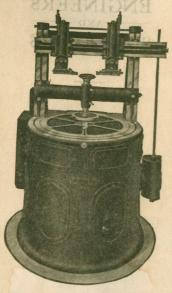
The most accurate circular dividing engine in the world and capable of dividing circles, each division of which is in its theoretical position to within one second of arc.
