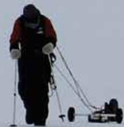
Snow accumulation measurement on the southern McMurdo Ice Shelf using radar. © Michelle Ryan.
