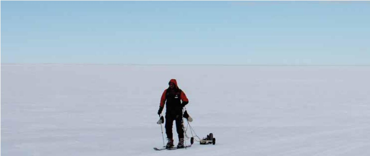
Snow accumulation measurement on the southern McMurdo Ice Shelf using radar. © Michelle Ryan.
