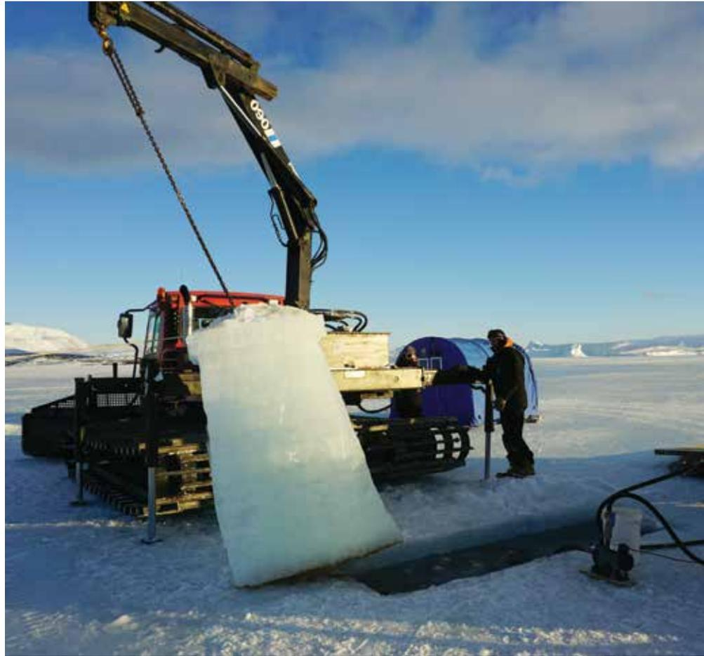
The K081 team used a hot water ice cutter and the hydraulic arm of the Scott Base vehicle to make the access hole for the underwater vehicles © Ian Hawes
