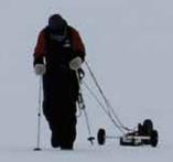
Snow accumulation measurement on the southern McMurdo Ice Shelf using radar. © Michelle Ryan
