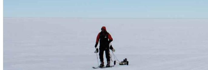
Snow accumulation measurement on the southern McMurdo Ice Shelf using radar. © Michelle Ryan.
