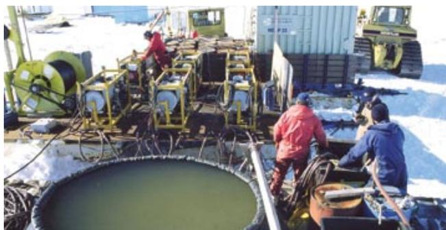
The ANDRILL site survey hot water drilling set up with flubber tank in foreground. *Miranda Huston Antarctica New Zealand Pictorial Collection KO42 02/03.*
