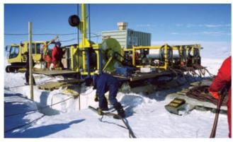
Testing of a hot water drilling system, which may be used in the ANDRILL scientific project. Environmental considerations are an integral part of planning for the multi-national project. *Miranda Huston Antarctica New Zealand Pictorial Collection K042 02/03*.
