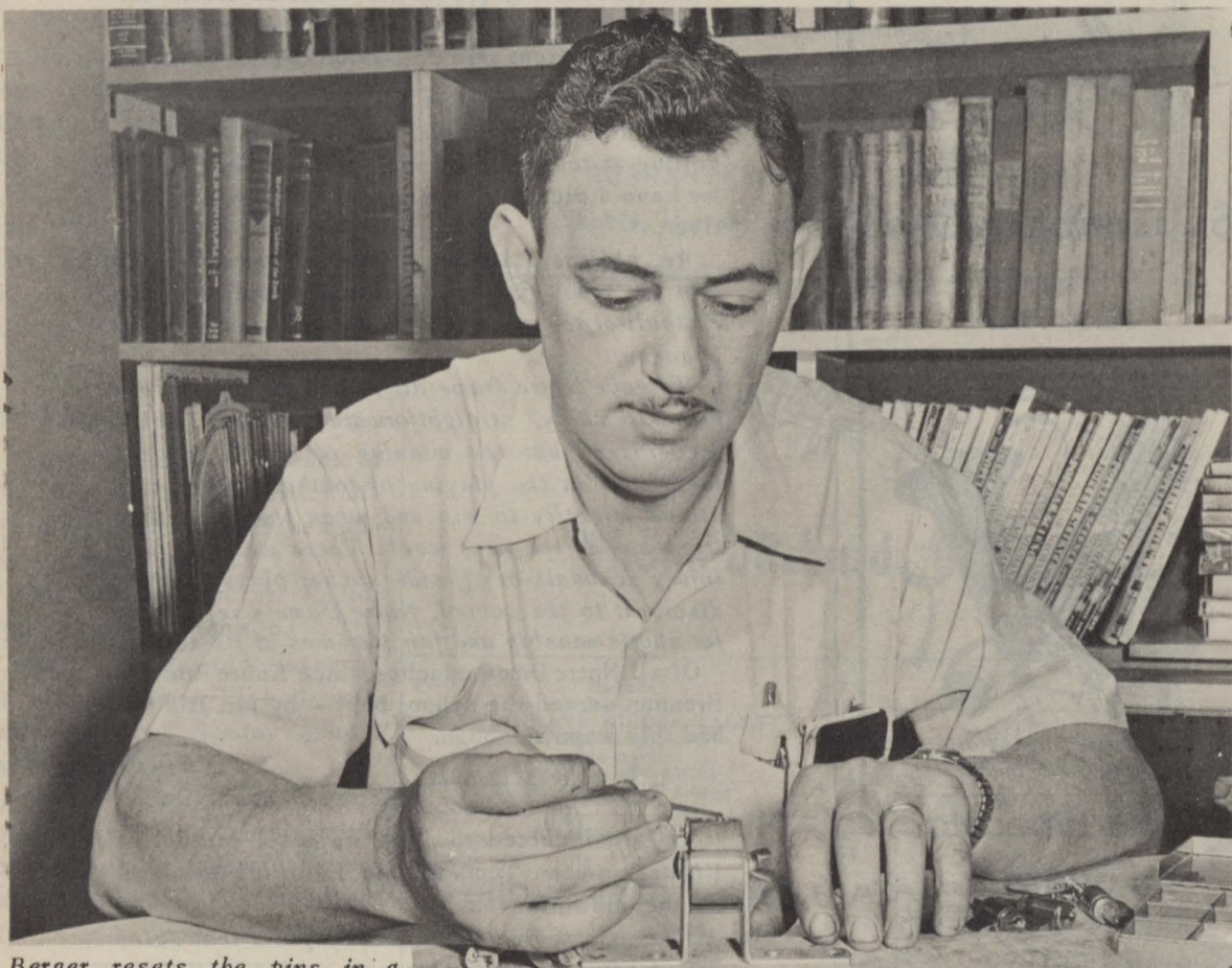
Berger resets the pins in a lock cylinder so it has a new combination. By this method, stolen or lost keys can be replaced without changing the entire locks on a house or business establishment.
