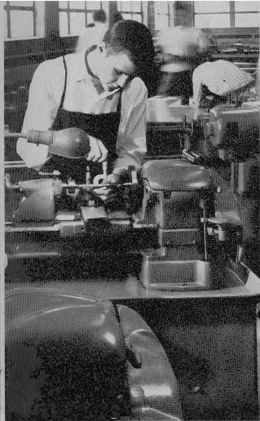
Making steel punches on the engine lathe, seniors Wayne Johnson and Bruce Peterson work in the metals shop.
