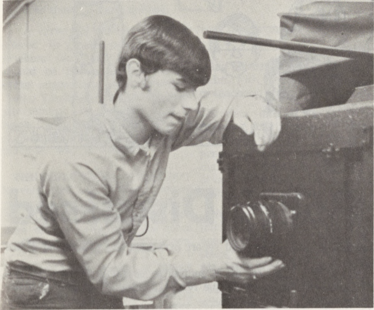
SECOND YEAR printing student Rich Reinwald, '69, adjusts the process camera lens in preparation for his next job.
