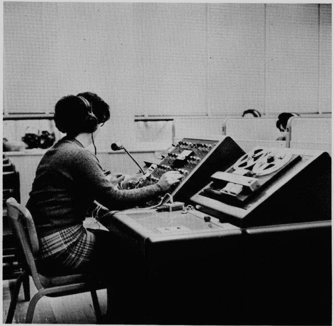
The control desk in the Language Laboratory enables Miss Fagan to listen to her pupils individually.
