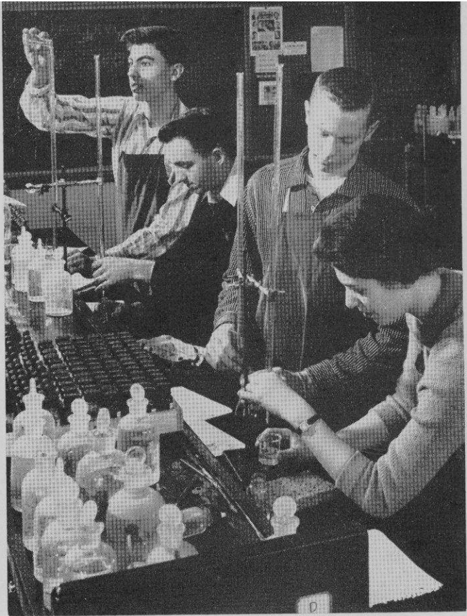
Alex Maurizi, Jay Doney, Jim Iverson, and Gail Braverman use Burette tubes to determine the percentage of solute in a solution of hydrogen chloride.
