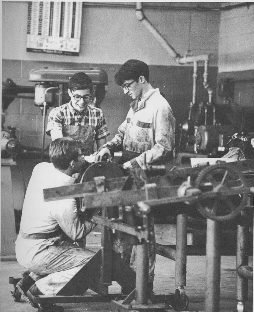
G. Davis, M. Stern, and S. Avella remove connecting rods to dismantle the engine they are working on.
