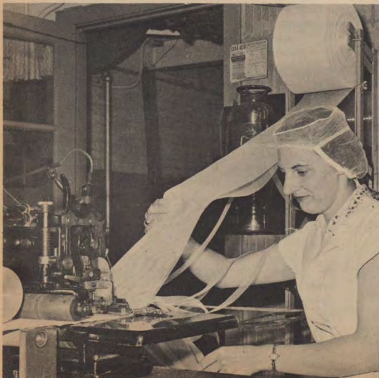
Another view of the material which filters out the tiny molecules of urea and waste products but which retains the big blood molecules and returns them, freshly "washed" to the patient.
