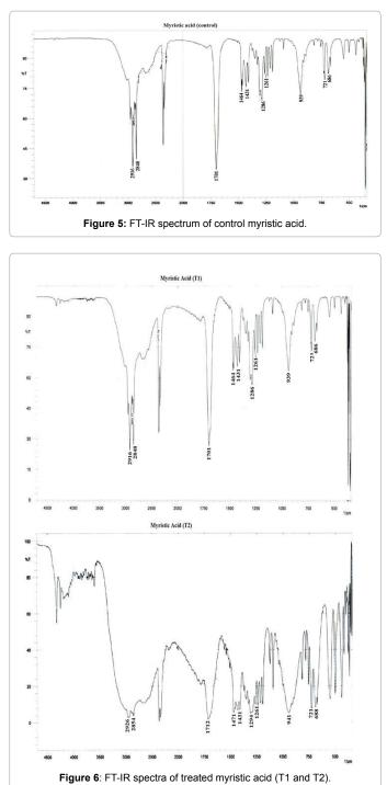
cm<sup>-1</sup> corresponded to C-H and C-C bending vibrations, respectively. The FT-IR peaks at 686, 721, and 939 cm<sup>-1</sup> were due to –OH swinging or rocking vibrations. This showed no significant difference in FT-IR peaks of control and T1 myristic acid sample.
