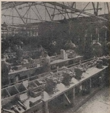
Fig. VIII. The running of assembly benches at right angles to the roof lights ensures that the light falls on the task without subjecting the worker to direct or reflected glare. Undesirable conditions would arise if employees were required to face directly into the roof-lights while working.
