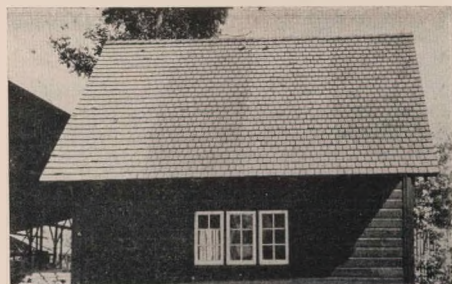
8. Roof of shingles treated in four different preservatives. Condition after three years' exposure Cupping of shingles treated in non-oily preservatives is clearly noticeable in the lighter coloured panels.
