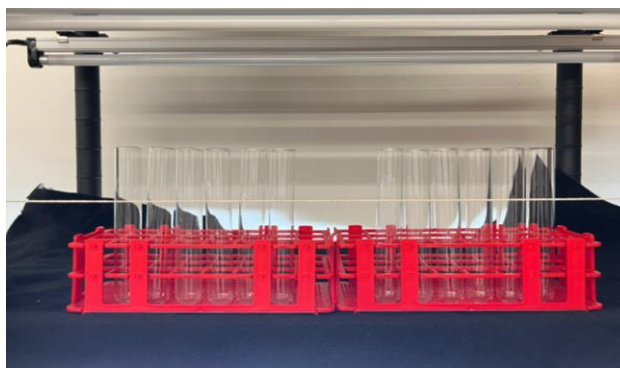
Figure 5: Experimental setup of test tubes. The arrangement of test tubes in the rack maximized the Daphnia visibility. Additionally, it displays the four 5 cm sections for recording vertical distribution.
