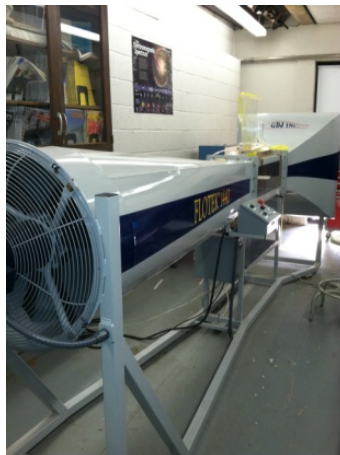
Figure 1: The Flotek 1440 Wind Tunnel.
