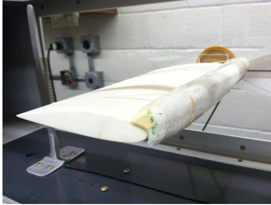
Figure 3: The glaze ice shape is attached to the leading edge of the wind tunnel.
