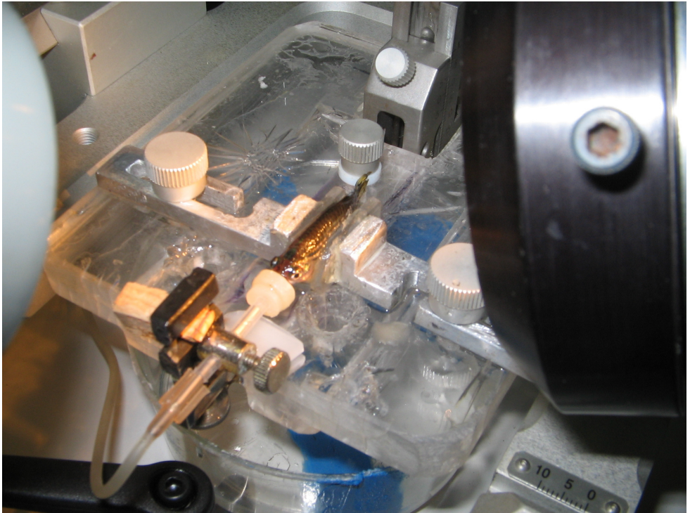
Figure 3: Close-up view of zebrafish mounted on stereotaxic apparatus.
