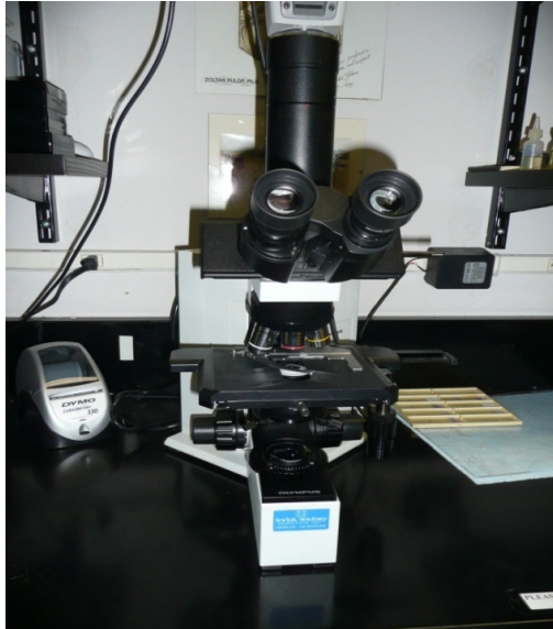
Figure 10: Olympus BX-40 Light Microscope with Sony ExWave HAD Sony Analog Camera using a FlashBus image capture card.
