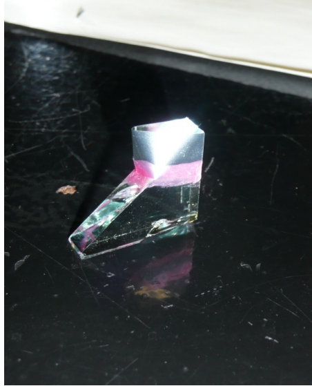
Figure 8: Picture of knife with a boat needed to slice 1\mu\text{m} semi-thin sections of tissue needed for light microscopy.
