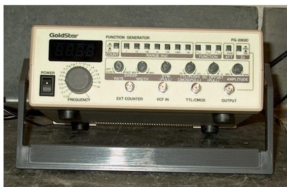
Figure 2: The function generator used to initiate the sinusoidally varying voltage.
