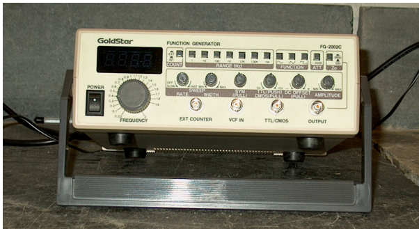
Figure 5: The function generator which produced the time-varying electric field.
