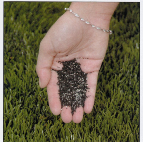
To cushion the surface grains of recycled athletic shoes, rubber, and soft silica are sprinkled between the blades of the turf.
