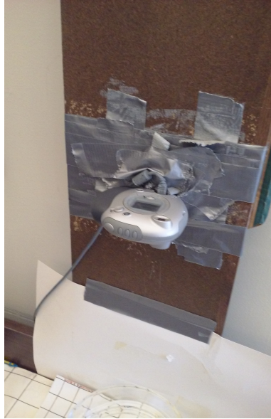
Figure 2: The video camera that was used in this experiment. The camera was attached to a wooden plank over a grid.
