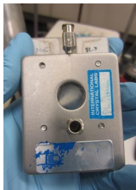
Figure 2. IR liquid transmission cell with a 0.1 mm fixed path length and NaCl salt plate windows. The fixed cell path length facilitated study of reproducible, dilute samples.
