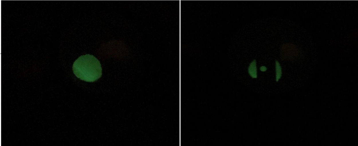
Figure 11: Electron Beam on Phosphor Screen. The electron beam unaltered out of the gun onto the phosphor screen (left) and a specimen, in this case a post on linear motion feedthrough with a hole drilled in it, dropped down in the path of the electron beam (right). In both images, the electron beam is not focused.
