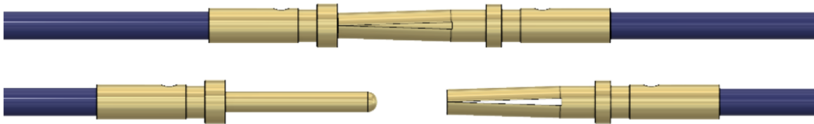
Figure 8: Quick-Disconnect. The figure above depicts the quick-disconnects that are located on the insulated conductors that make connections between the feedthrough and the gun. The disconnect feature includes a male pin and female socket that coincide when connected.
