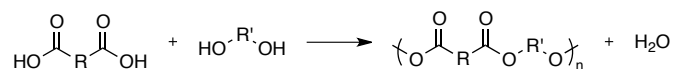
Scheme 1. General step-growth polymerization of a diacid and diol through the extrusion of water.
